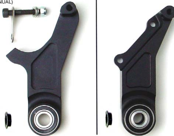
DHS BRAKE ARMS: HAYES (MC74) ON LEFT AND SHIMANO (ISO 8" ROTOR) ON RIGHT
