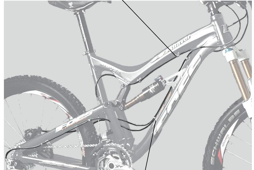
Down Tube Cable Guides 1: for Rear Derailleur Cable 2: for Rear Disc Brake line
